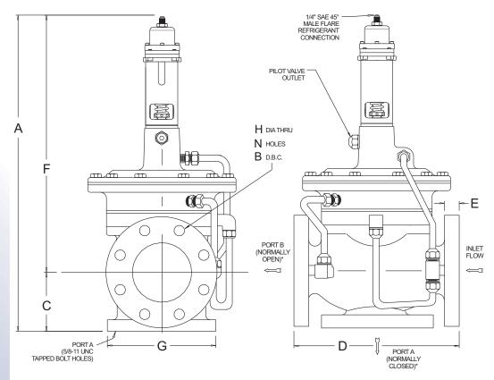
\*NOTE: Normally closed valves open on pressure increase, normally open valves close on pressure increase.
